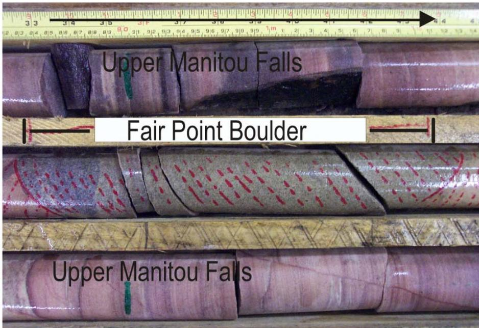
Figure 11. Unconformity above the Fair Point Sequence: a) red saprolite between the Fair Point (Jackfish Basin) and Upper Manitou Falls (part of the William River Basin) sequences, at a depth of 110 m in drillcore FC-071; core boxes are 70 cm long; b) Fair Point boulder reworked into the base of the Upper Manitou Falls Sequence, at a depth of 232 m in drillcore MT-02, north of Net Lake trend; boulder is 12 cm wide.
