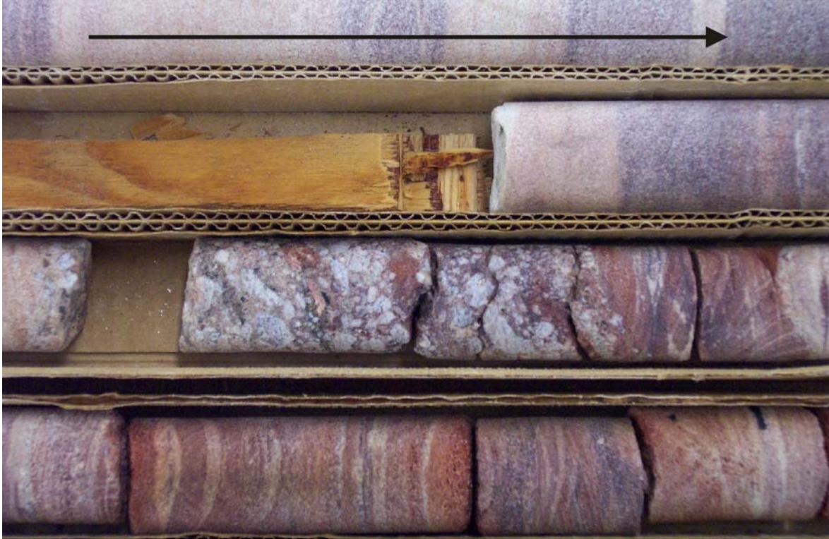
**Figure 2. Massive conglomerate lag above the unconformity between the Upper Manitou Falls and Lower Wolverine Point sequences, at a depth of 186 m in drillcore FC-052, east of Maybelle River; lag is 15 cm thick; arrow indicates stratigraphic younging direction.**
