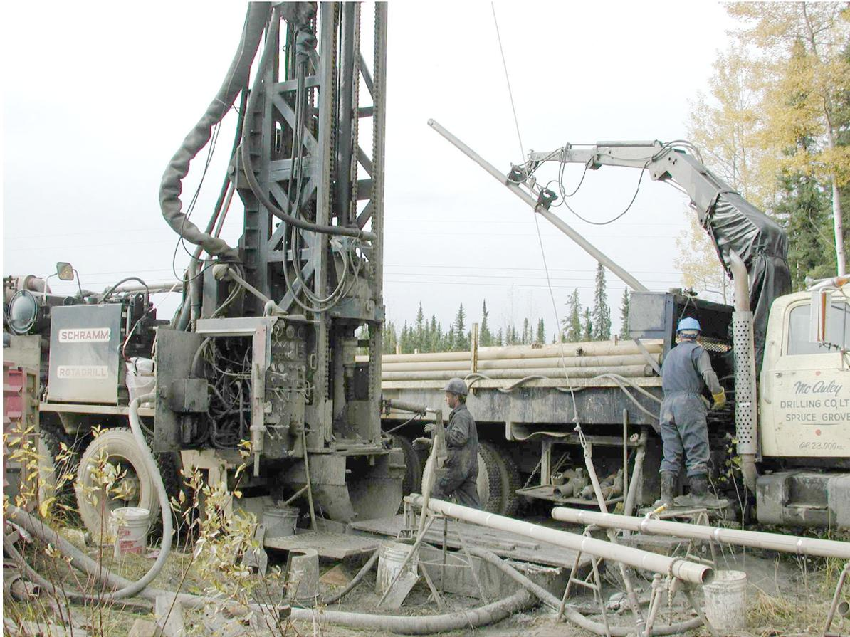
Figure 17. Wet-rotary coring rig.
