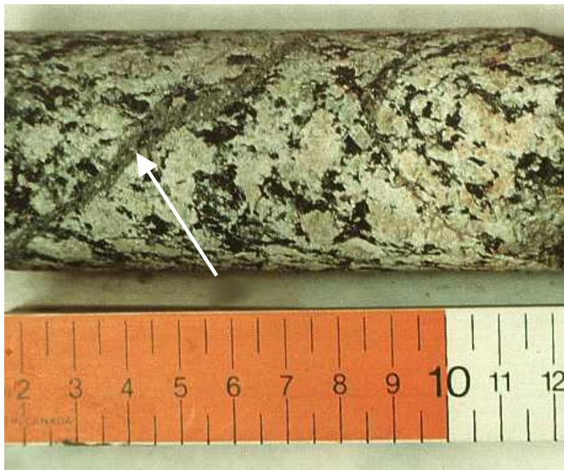
Figure 12. Basement granite-gneiss with a fracture infilled by rock dust (arrow), 375.6 m in drillhole ST003. Scale marked in centimetres.
