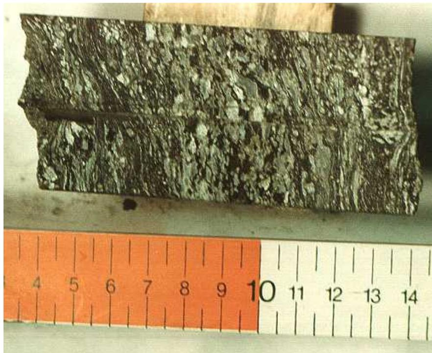
Figure 10. Vitrified (sintered) granite with flow textures, 335.8 m in drillhole ST003. Scale marked in centimetres.
