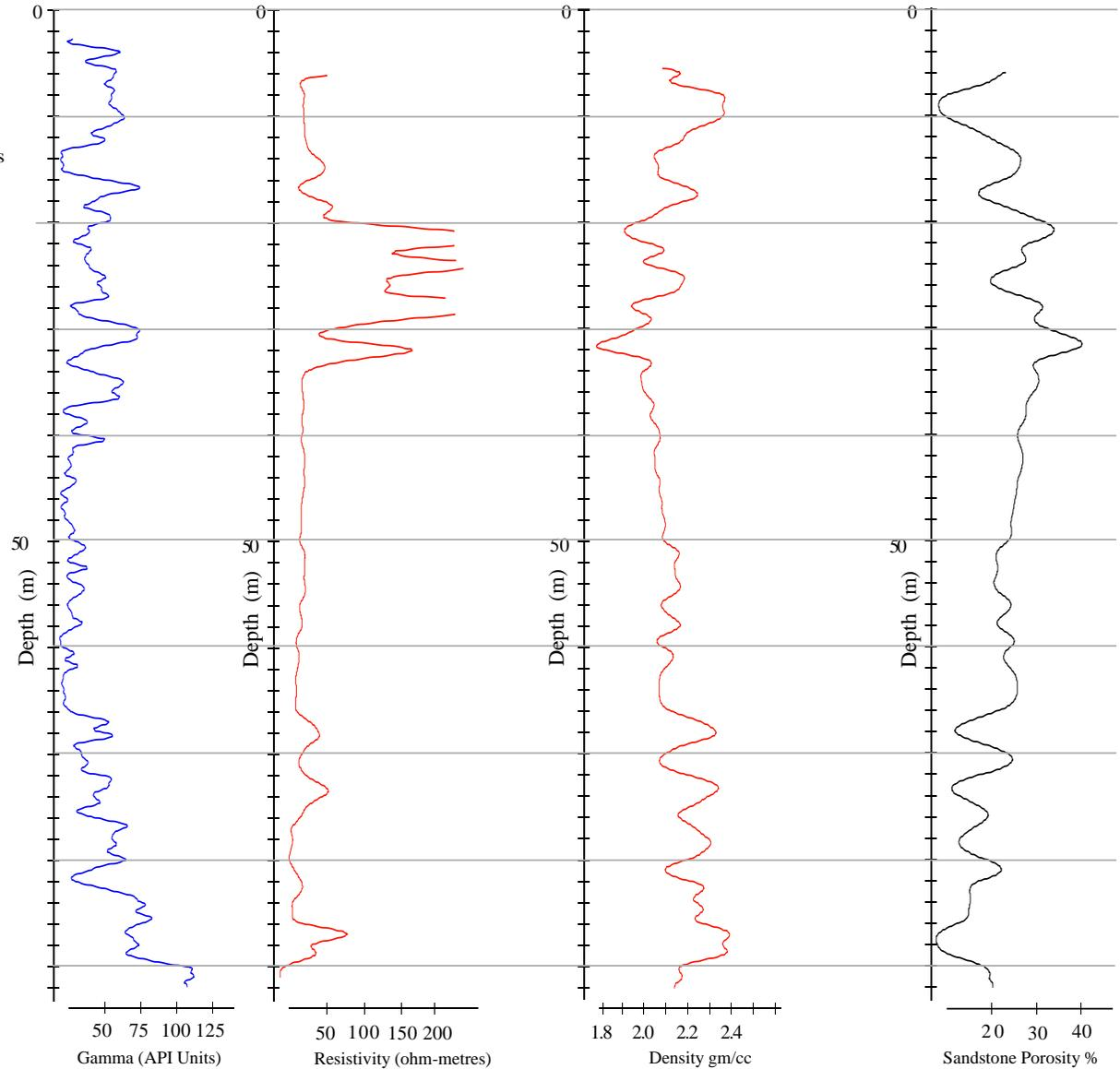
Figure A2-10. Lithological and downhole geophysical properties of Quaternary sediments in borehole UTF96 water supply well (UTF96-WSW).
