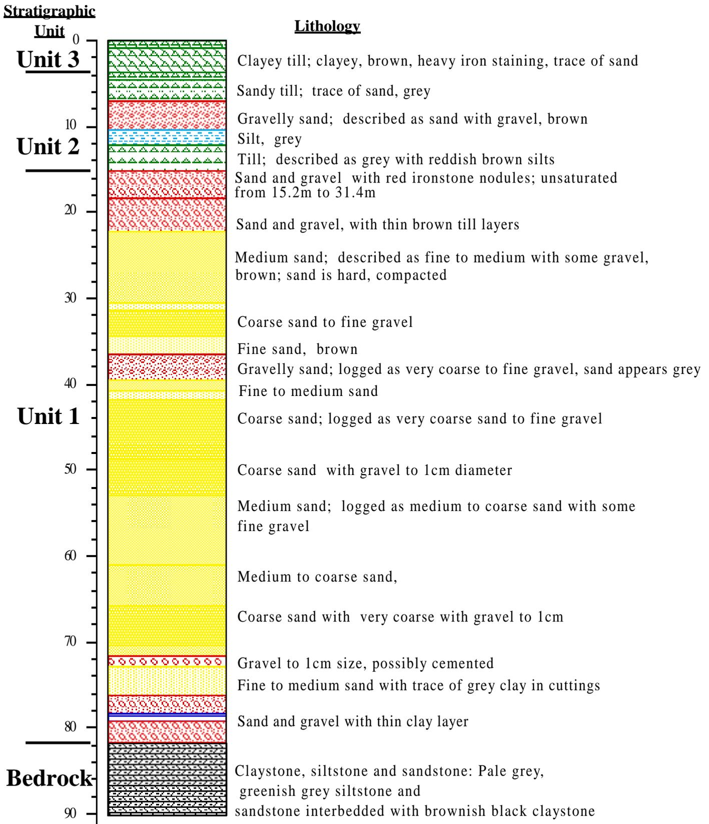
Figure A2-9. Litholog of borehole WW1.
