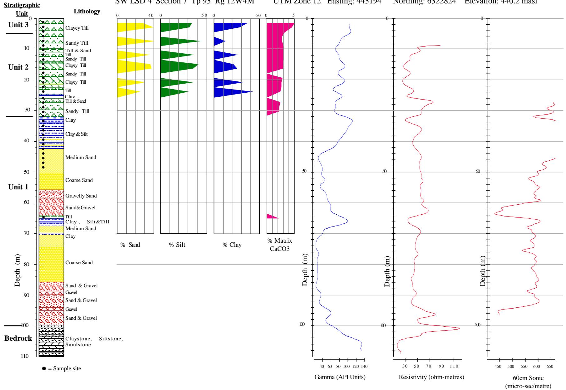
Figure A2-5. Lithological, mineralogical, and downhole geophysical properties of Quaternary sediments in borehole UTF96-2.
