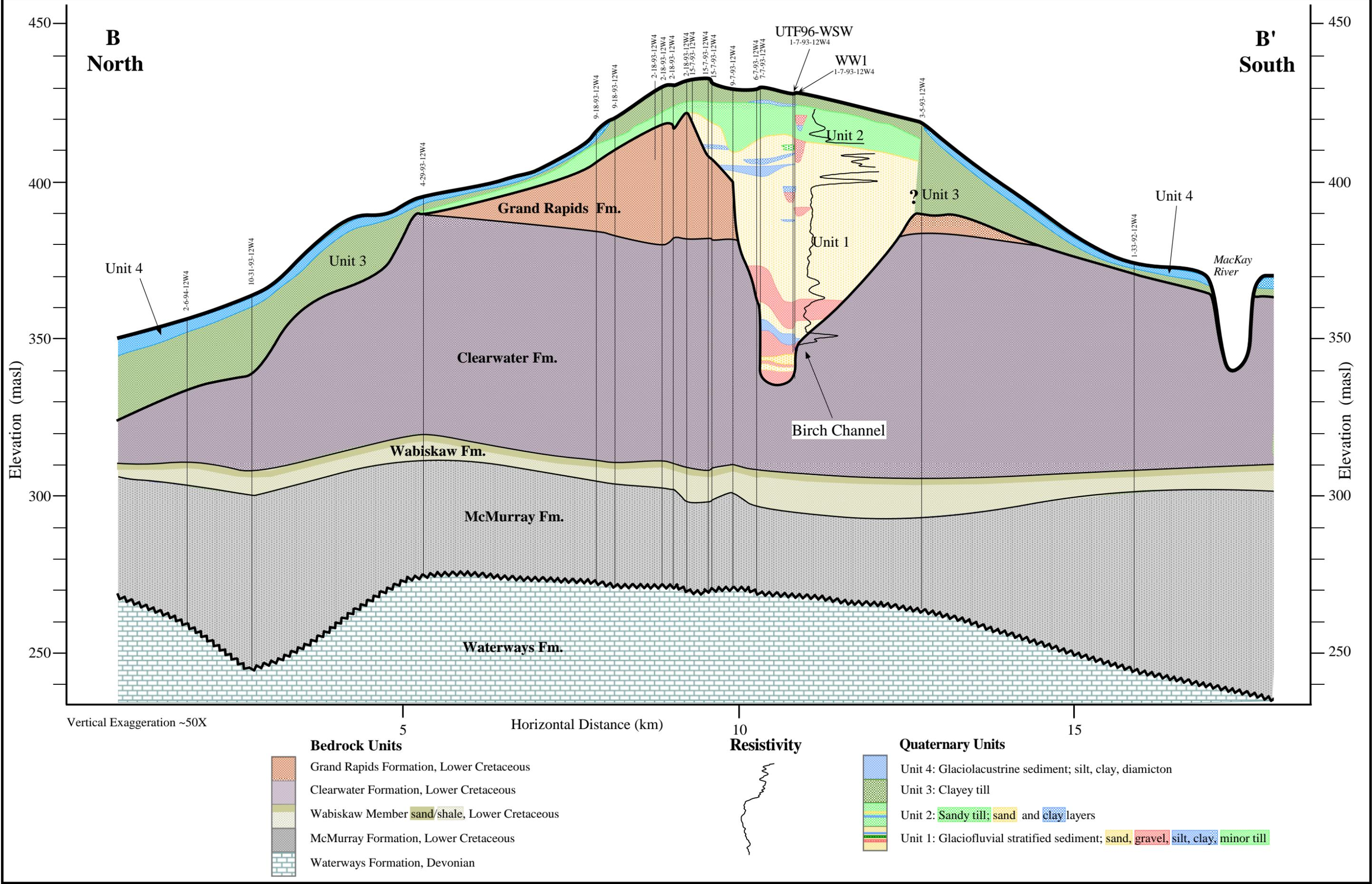
Figure 6. Geological cross-section B-B' across the Birch Channel.
