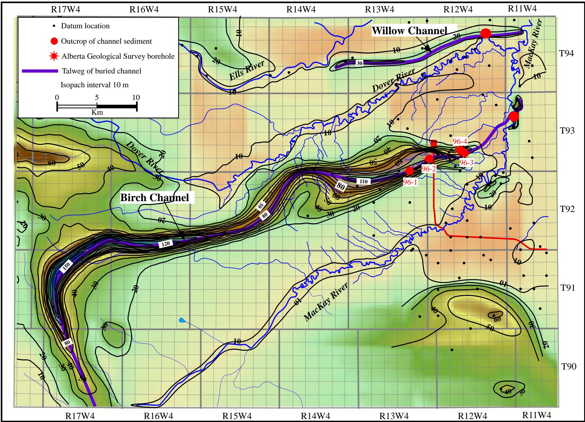
Figure 7. Thickness of Quaternary drift above bedrock.
