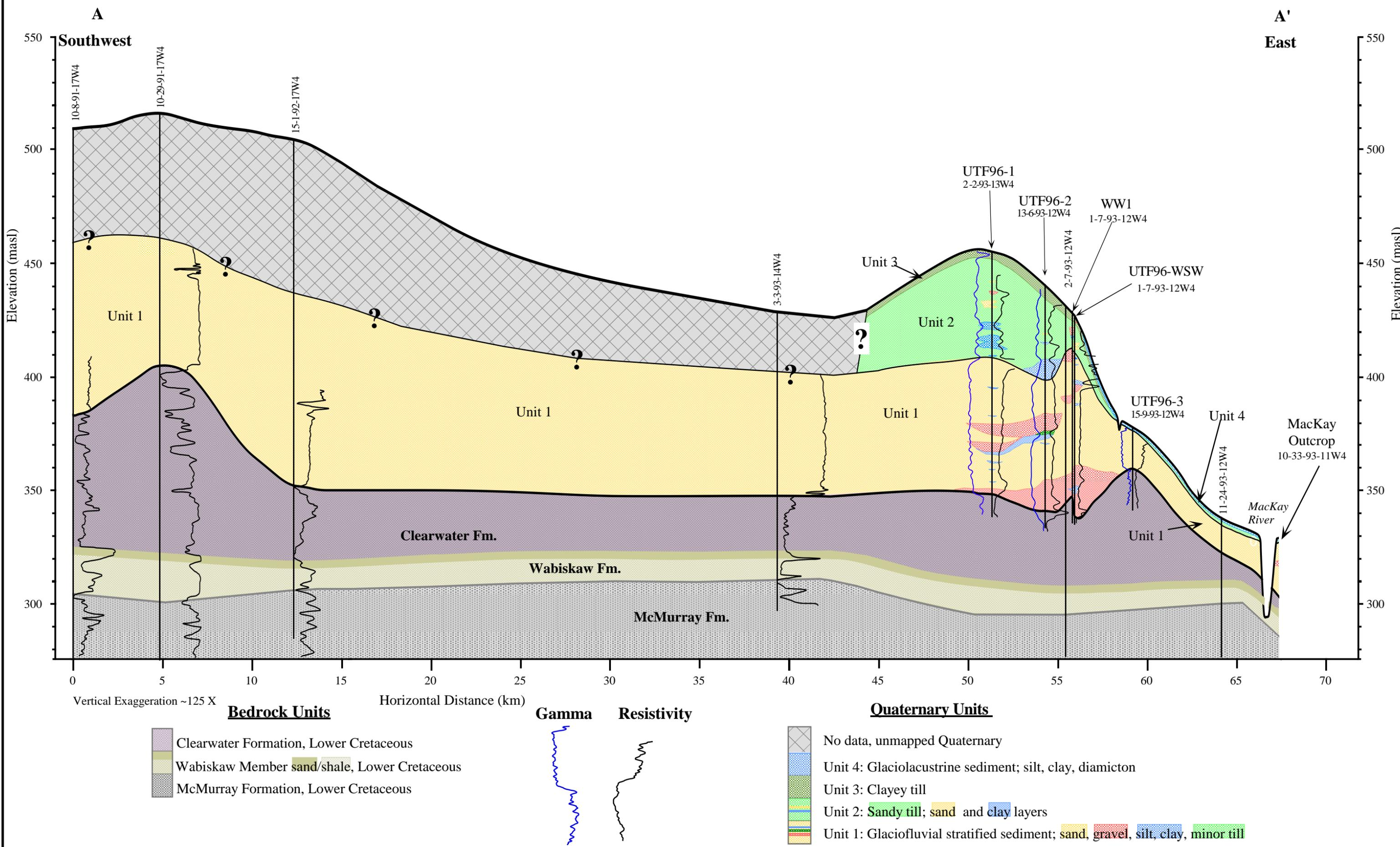
Figure 5. Geological cross-section A-A' along the Birch Channel.
