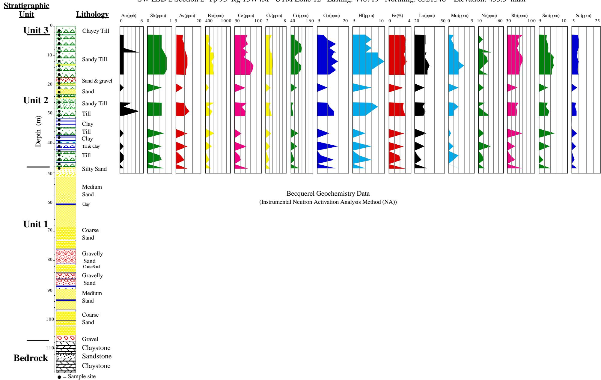
Figure A2-11. Geochemical analysis of the silt-clay fraction of tills, borehole UTF96-1.
