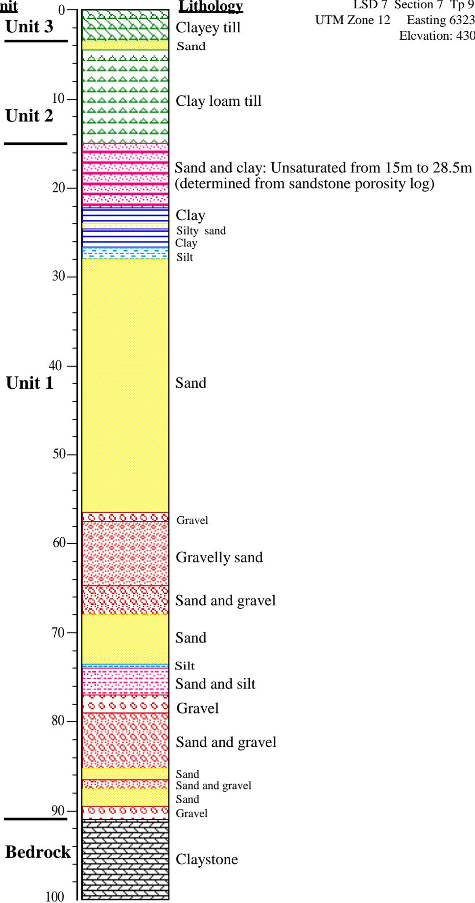
Figure A2-8. Litholog of borehole WDW3 Dover.
