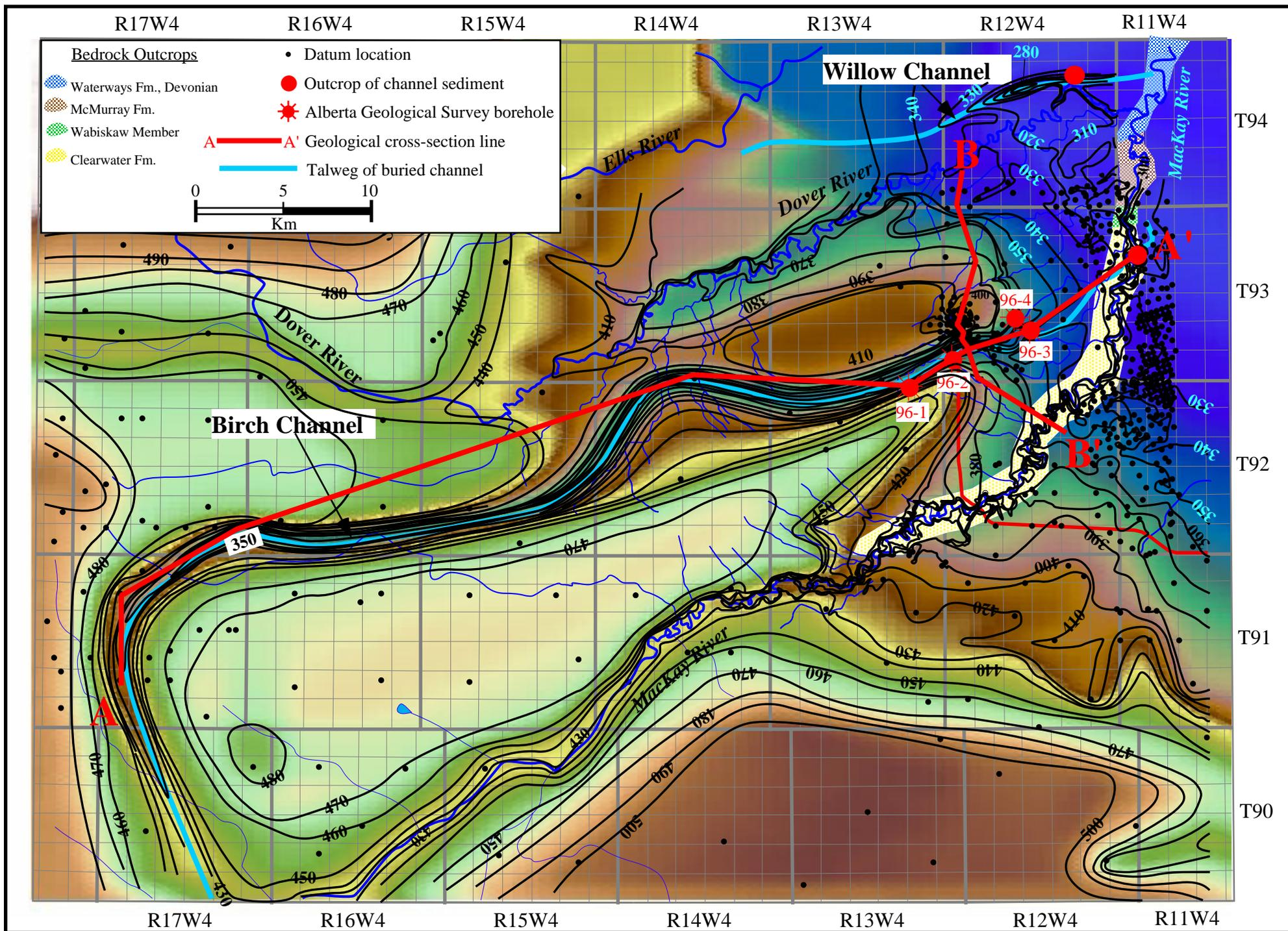
Figure 4. Bedrock topography and talwegs of buried channels.
