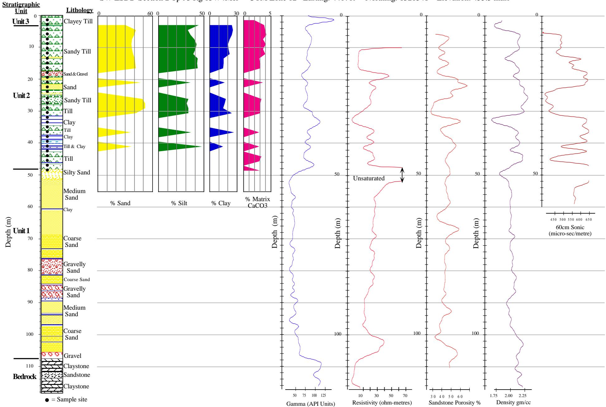
Figure A2-4. Lithological, mineralogical, and downhole geophysical properties of Quaternary sediments in borehole UTF 96-1 .
