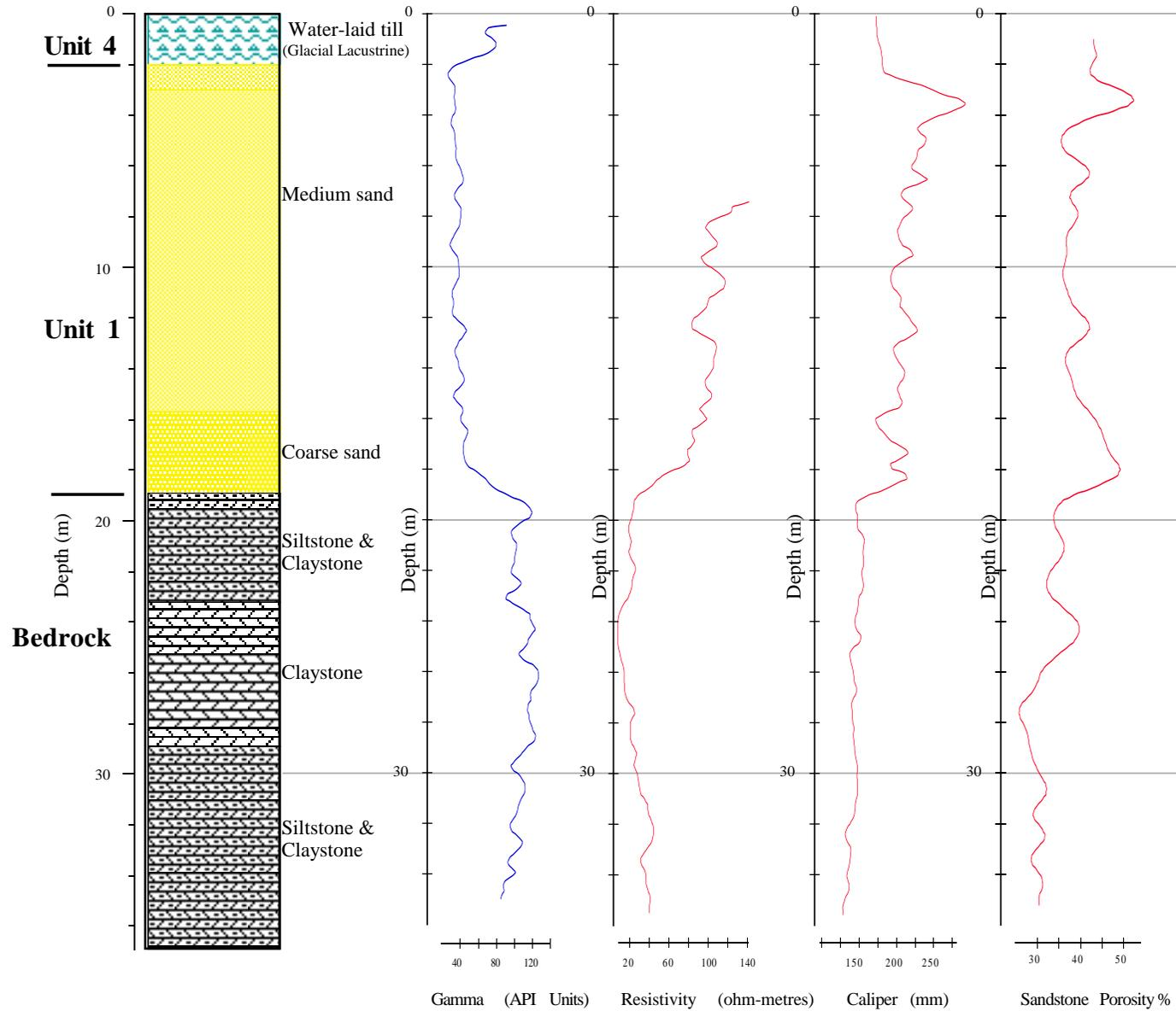
Figure A2-6. Lithological and downhole geophysical properties of Quaternary sediments in borehole UTF96-3.
