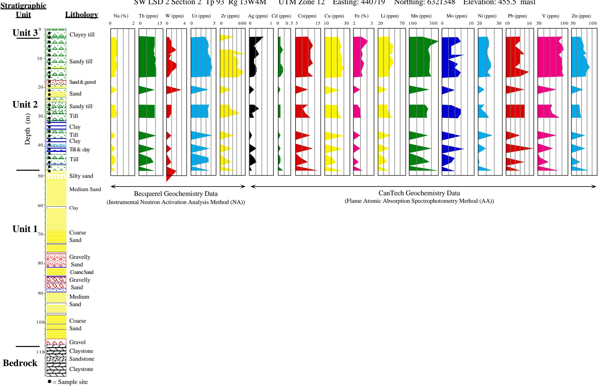
Figure A2-12. Geochemical analysis of the silt-clay fraction of tills, borehole UTF96-1.
