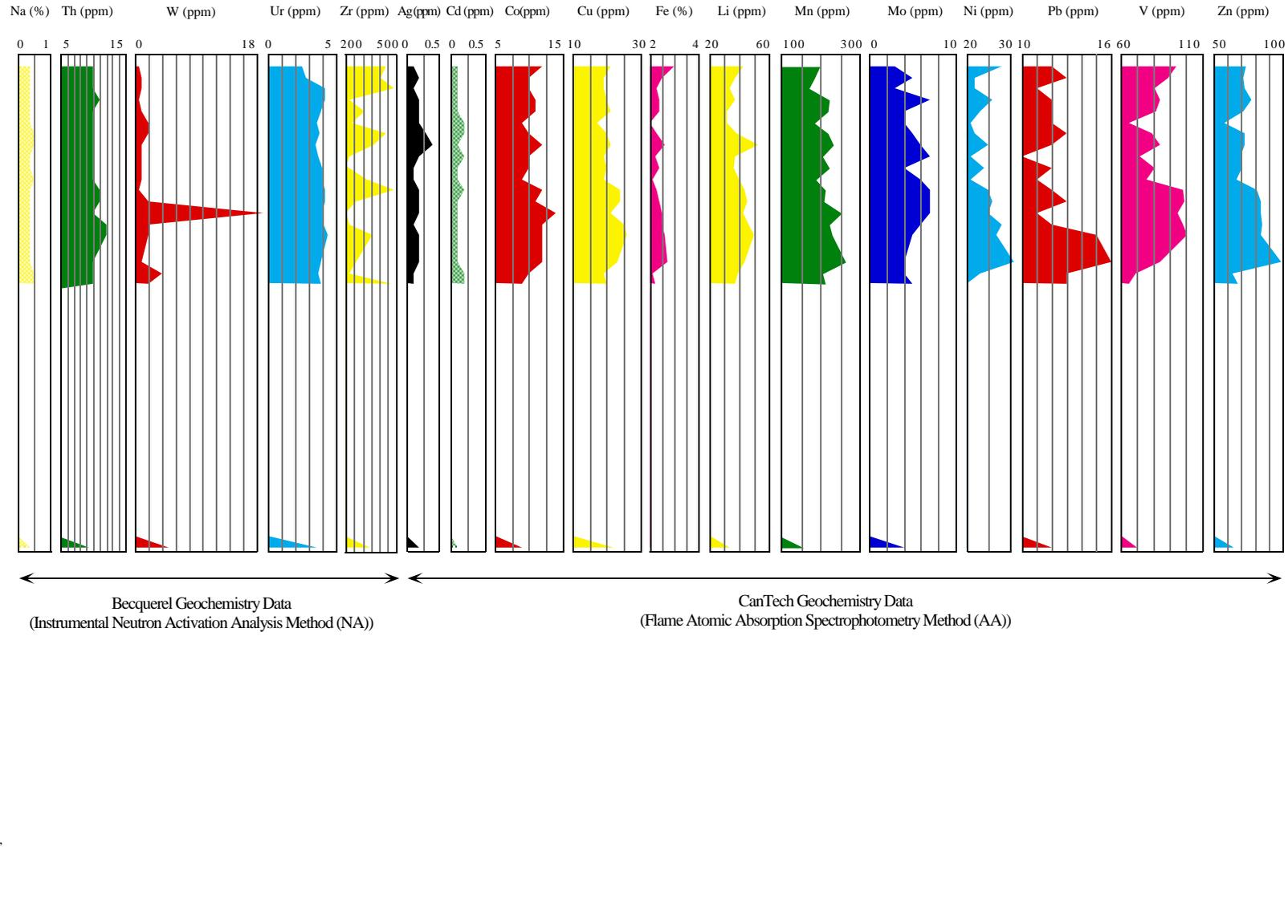
Figure A2-14. Geochemical analysis of the silt-clay fraction of tills, borehole UTF96-2.
