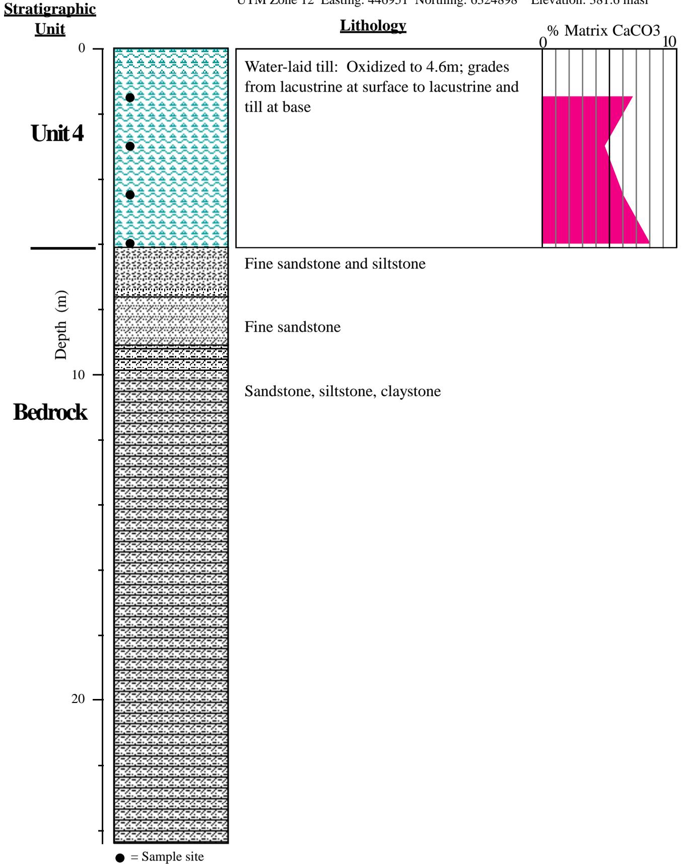
Figure A2-7. Lithological and mineralogical properties of Quaternary sediments in borehole UTF96-4.
