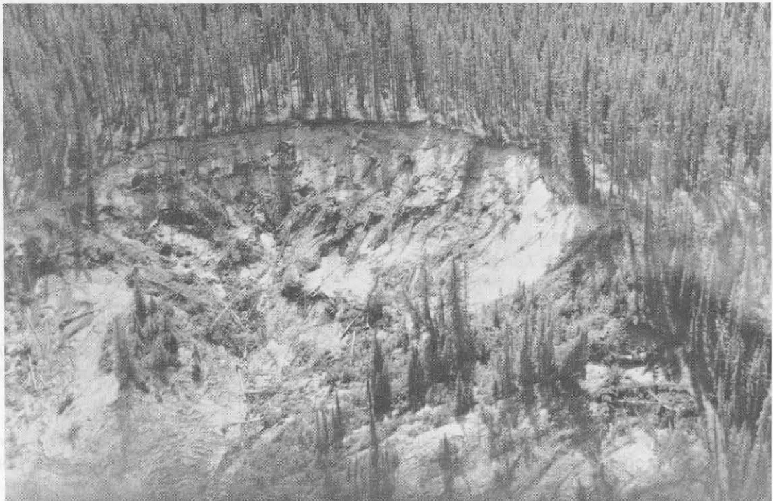
PHOTO 8. Large slide in glaciolacustrine silts and clays caused by groundwater discharge near Wildhay River. (Township 55, Range 25)
