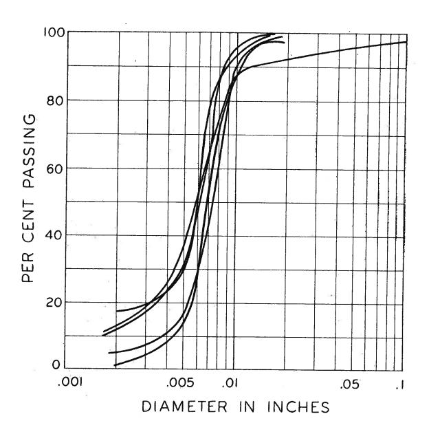
Figure 1. Size analyses of typical quicksand aquifers
