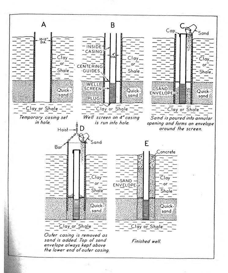
Figure 2. Construction of a gravel envelope well by the pull-back method
