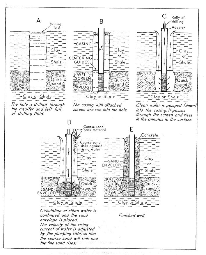
Figure 3. Construction of a gravel envelope well by the "flush-in" method
