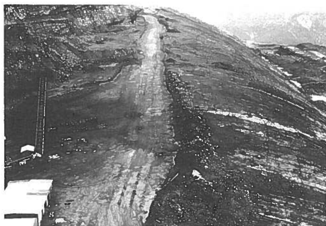
Figure 11. Exposure of the footwall of the No. 4 coal seam along the McEvoy Anticline in the No. 9 Mine. The view is along the fold axis in southeastern direction.
