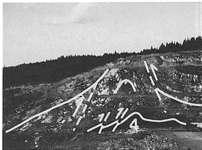
Figure 23. Structural thickening of No. 4 coal seam and accompanying hinge collapse along the McEvoy Anticline in the No. 9 Mine, resulting from hinge dilation in a chevron fold.
