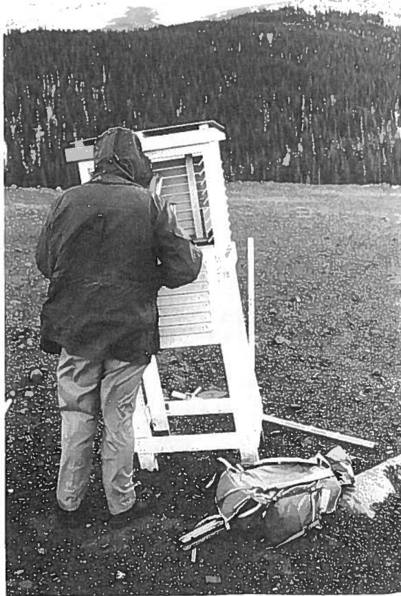
PLATE 13. Displacement of screen support from vertical.
