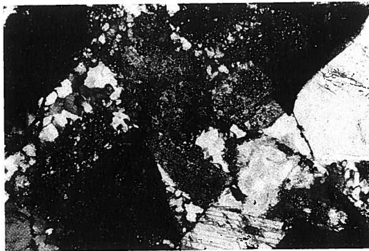
FIGURE 2. Figure 1, above, crossed nicols, showing the anhedral cherty texture of the intergranular quartz. Chert cement is rare in most phases of the Blairmore and Mannville sandstones.
