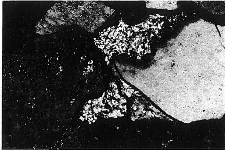
FIGURE 2. Figure 1, above, crossed nicols. Note the small patches of authigenic illite in plagioclase grain to the left.
