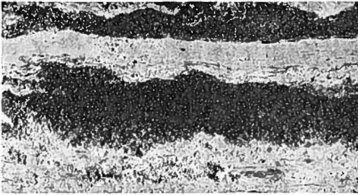
FIGURE 1. Minor structure in laminated silt of the McMurray Formation showing regular laminae of oil sand (dark color) and silt. Magnification X2.5.
