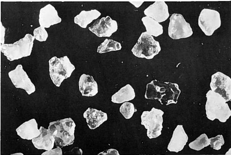
FIGURES 1, 2. Photomicrographs of two fine-grained sands showing mixture of angular and rounded particles in the McMurray Formation. Magnification X27.
