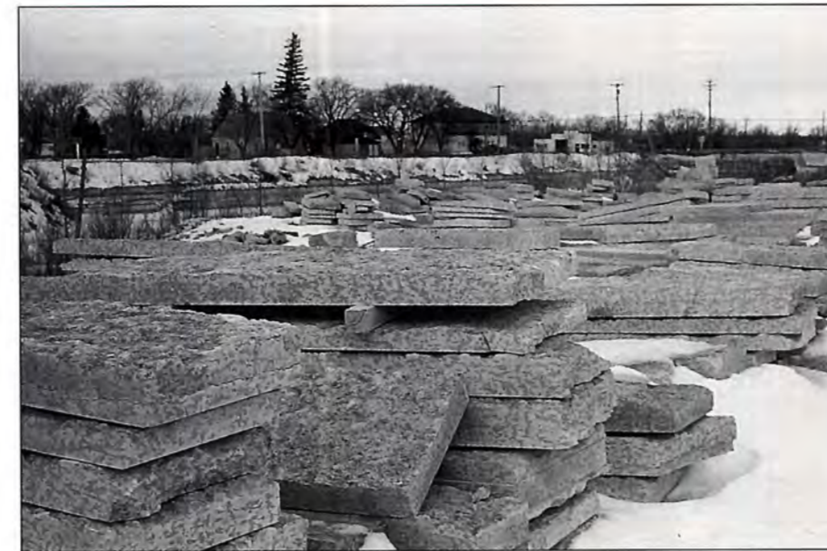
Figure 9.29 Tyndall Limestone building stone, burrow-mottled carbonates of the Red River Formation, Gillis Quarry, Garson, Manitoba; four by four inch staves provide scale. Photograph R.K. Bezys.
